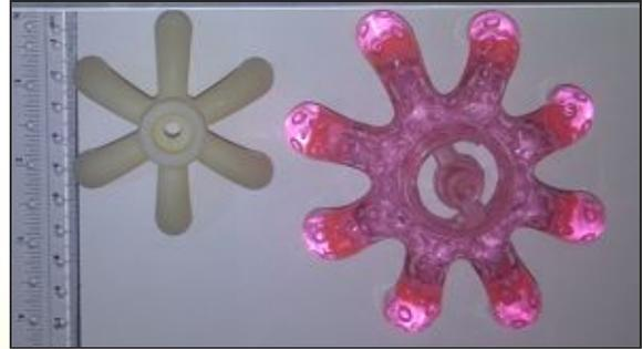
After the molds were made, we needed to decide what kind of plastic to use for production. Avela prototyped two kinds of plastic for the LumpBuster and Ashley put several into the field for testing. One plastic proved strong but to brittle for aggressive use. We chose a more flexible plastic for the final production. We developed quality control (QC) procedures and went into final production.
